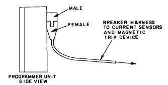
Fig. 2. Normal In Service breaker connection
